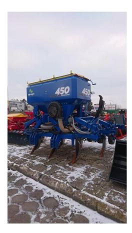
Figures 1,2,3: GB Hybrid, hybrid subsoiler and strip-till combination
