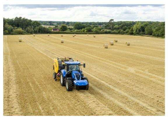
Figure 3: METHANE POWER TRACTOR in the field
