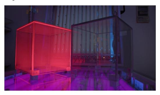
**Figure 5:** Demonstration of the nanocoating effect when two cubes of coated and uncoated glass are illuminated by UV light.
