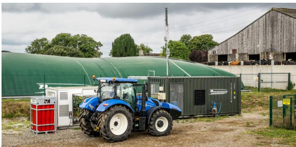
**Figure 1.** Methane capturing system on 100 dairy cow farm powering a New Holland T6 180 methane tractor (copyrights New Holland).
