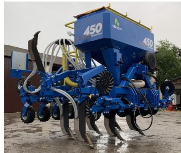
Figure 2: GB Hybrid- Strip-till and subsoiler
