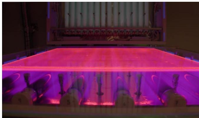
**Figure 1:** Glass covered with Brite's nanostructured coatings, illuminated with low-power UV light.
