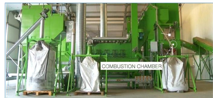
**Figure 1:** Fluidized bed combustion process maximizes poultry manure combustion efficiency and minimizes emissions
