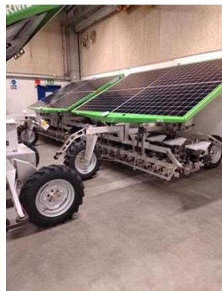
**Figure 1 and 2:** FarmDroid electrically powered field robot with solar panels
