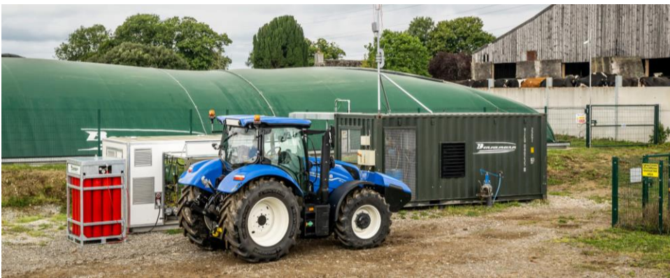
Figure 1. Methane capturing system on 100 dairy cow farm powering a New Holland T6 180 methane tractor (copyrights New Holland).
